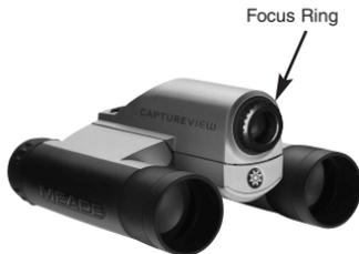
**Note:** The Binocular focus knob does not affect the camera focus. The camera's focus is determined by the Focus ring setting:
